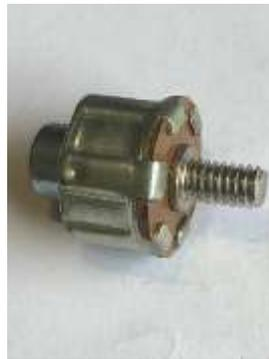
(see photos). This fuse is peculiar to the lighter, is part #14429 and is listed for all three years of T-Birds and other Ford models from 1952 upward. Some of these fuses have a small hole in the rear to reset the fuse with a pin or paper clip wire. Since reproduction lighter elements are reported to draw near 7 amps in 6-volt applications and 8 amps in 12-volt systems the use of an in-line fuse of at least 10 amps would be wise if one does
