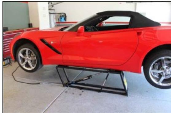
“With a three inch collapsed height, the QuickJack can get in where other jacks only wish they could. And without any cross members, you can match frame positions to almost any vehicle width.” For more information and prices for the BL- 5000SLX go to the QuickJack website at <https://www.quickjack.com>.” I recently purchased the BL-5000SLX and will report on its use with my T-
