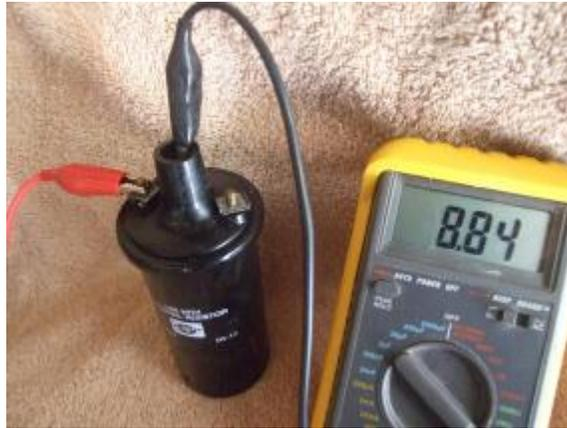
3 – This reading of 8.84 does indicate that the coil's secondary windings are not putting out as much voltage as they should; the minimum acceptable resistance reading here should be 11.00, with approximately 13.5 being normal.
