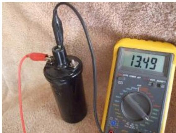
5 – Ah, yes – 13.49 is more like it. Now there should be plenty of fire in the hole! All that remains is to put it back in the car, connect the leads to the terminals, plug in the distributor cable and start her up!
