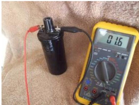
4 – Here's the primary reading on the replacement GM Delco coil. The 1.6 reading is exactly what it should be but, again, the real telling is what the secondary resistance reading is.
