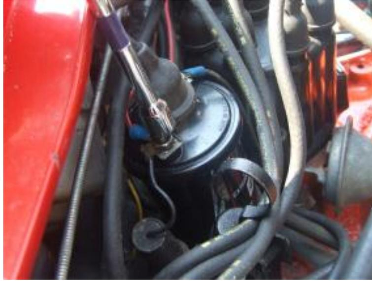
**1** – Use a nut driver or a small wrench to loosen the securing nuts on the coil terminals and remove the leads; the positive side of the coil has a condenser lead attached in addition to a positive lead. Then loosen the bottom clamp screw, pull out the center cable that goes to the distributor and remove the coil. Alternatively, you can check the coil right in the car with your multimeter if you remove all three leads first.
