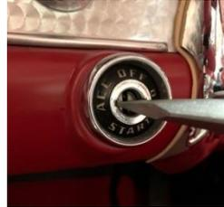
ignition switch from the dash and let it hang. Attach a jumper wire to the “Bat” terminal of the switch; this terminal will
