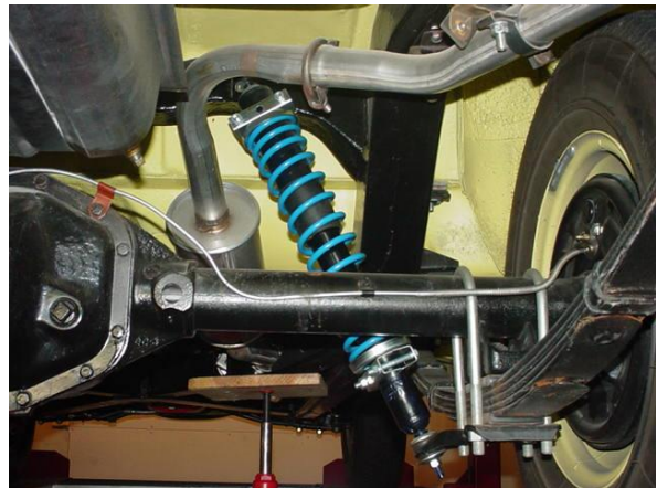
Shock Absorber shown with blue overload spring installed.
