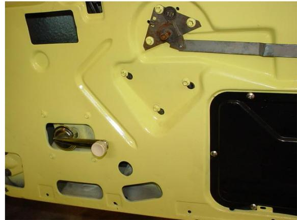
After tightening the screws restore the upper limit bracket to its original position. Now try out the window. By changing the position of the scissors you have increased the upper travel limits of the mechanism. This worked for me and I did not have to remove the glass or any of the mechanism to accomplish the modification.
